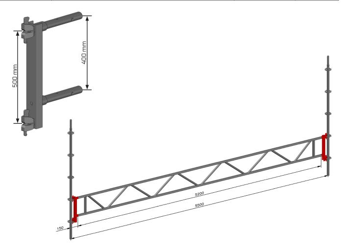
With sufficient load-bearing capacity of the connected structures (bridging and /or support), each adapter for lattice girders enables a vertical shear capacity Fv = 20 kN. The value refers to the characteristic value of the effect (service/working load).
