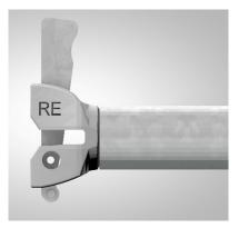
By optimizing the wedge head geometry, an increased load capacity of the ledgers is achieved. This is caused by modifying the height of the wedge heads, without limiting the introduced characteristics of the scaffolding system. All wedge heads of ledgers, transoms and vertical braces, as well as all wedges have received an additional hole in the lower area. The holes of the heads and wedges
